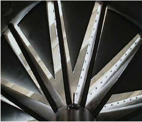
Air assist flare designs (Images courtesy of © John Zink Company LLC)
