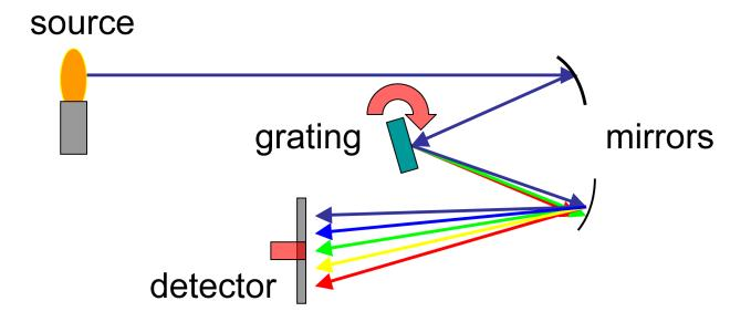
Figure 1: Schematic of optical spectrometer. (Source: <u>Wikimedia Commons</u>. Full credit to Wikipedia User: Kkmurray. This file is licensed under the <u>Creative Commons</u> <u>Attribution-Share Alike 3.0 Unported</u> license. No changes have been made to the original file.)
